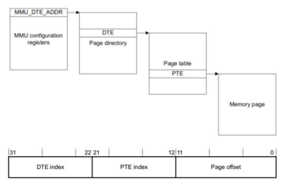
32bit address structure, the first 10 bits of the first-level page table offset, the middle 10 bits of the second-level page table offset, and the last 12 bits within the page offset.
