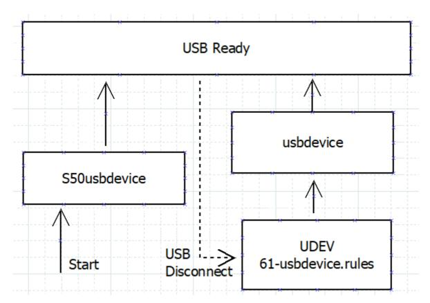
You can directly modify .usb\_config and execute S50usbdevce script to configure USB function when needed.
