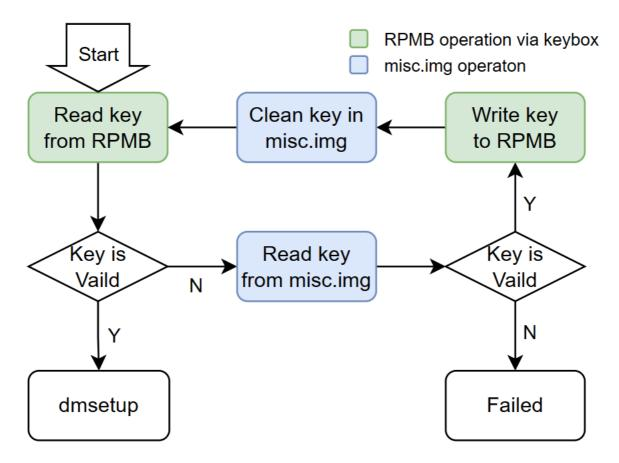
In the diagram, operations for reading and writing keys from RPMB are all performed through the KeyBox software. Additionally, certain runtime restrictions have been implemented to prevent KeyBox from being extracted from the Ramdisk for unauthorized use. For example, it must run within a program with PID=1 and must be executed in the Ramdisk. For more details on KeyBox, you can refer to the KeyBox section.
