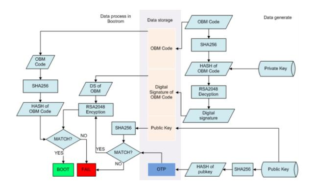
The above flowchart illustrates the process of Bootrom verifying the loader, and the verification process for other firmware is similar.
