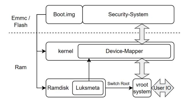
The above diagram roughly illustrates how boot.img verifies or decrypts the system:
