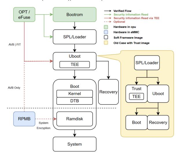
Note: The Trust firmware is at the same level as the Uboot firmware, both verified by SPL or Loader, following the same verification process as Uboot. On new chip platforms, the Trust firmware has been integrated into the Uboot firmware.
