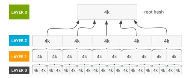
Root-Hash first verifies the Hash-Map to ensure its accuracy, and then a virtual partition is created through Device-Mapper-Verity and mounted . When using the partition, Kernel performs hash verification separately for the 4K partition where the access I/O occurs and compares it with the Hash-Map. When an error is detected during verification, it returns an I/O error, similar to symptoms of filesystem corruption.
