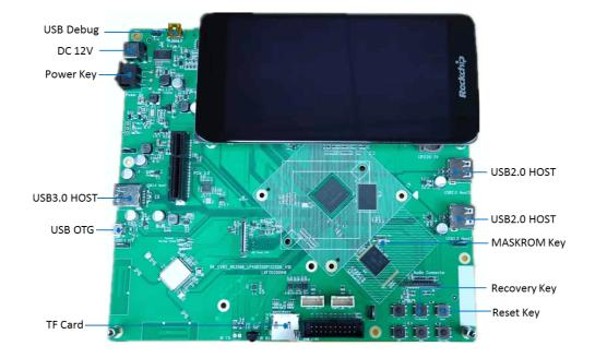
The interface distribution diagram for RK3568 EVB1 development board is as follows:
