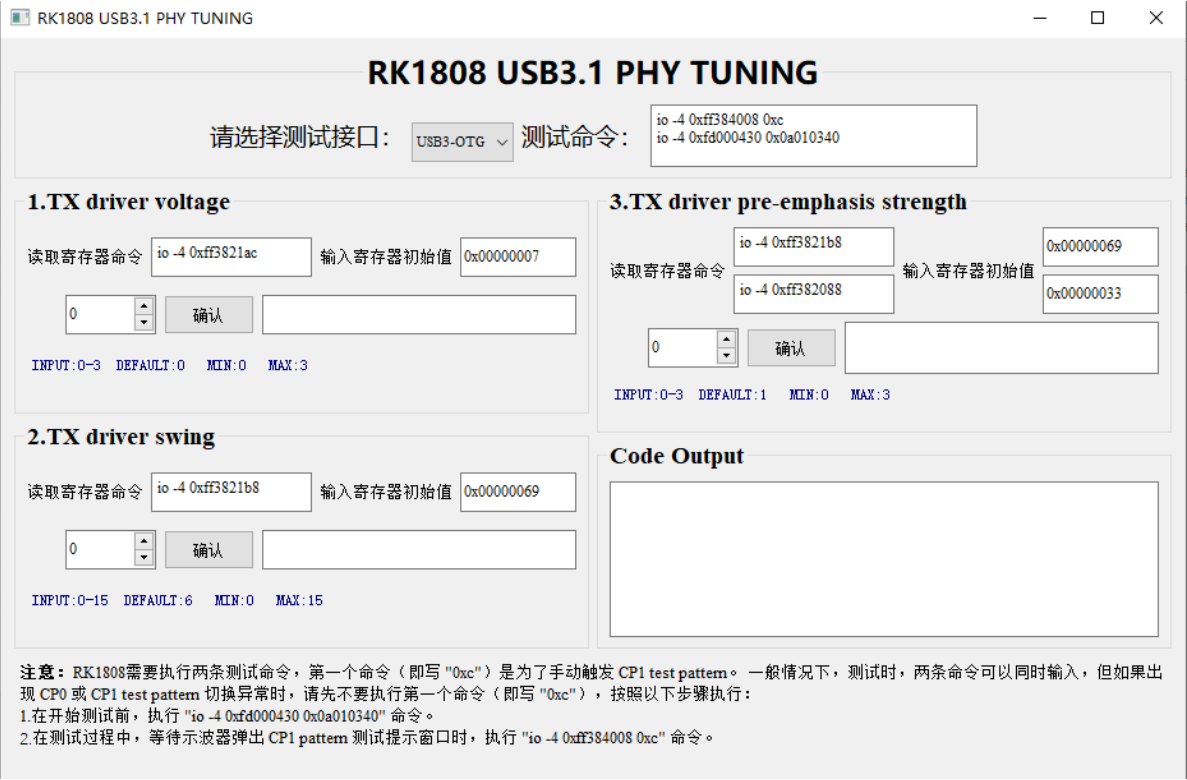
图9 RK1808 USB3.1 PHY Tuning Interface
