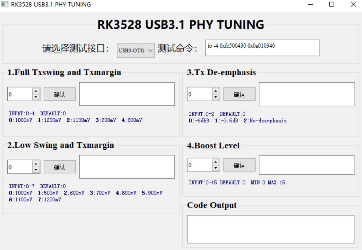
图11 RK3528 USB3.1 PHY Tuning Interface
