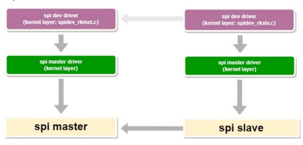
The purpose of providing "SPI Slave Software In Kernel" is to provide reference for protocol and device drivers, and the end customer should also define their product requirements on the application buffer of the slave end to achieve business.
