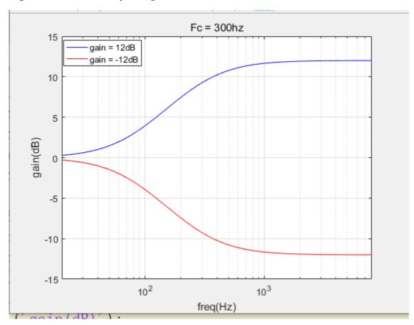
The figure below shows an example of low-shelf filter which Fc = 1000Hz,Gain =  $\pm 12$ :
